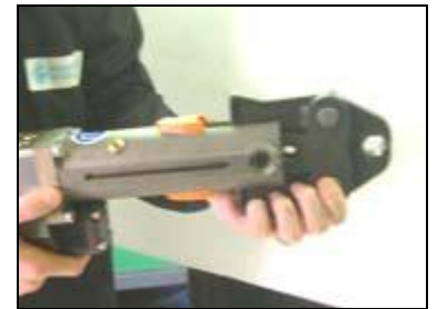
F. Insert the appropriate jaw into the pressing tool and push in holding pin until it locks into place.
