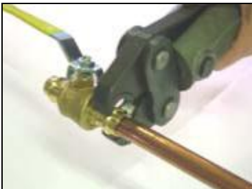
G. Open the jaw and place at right angles on the fitting. Visually check the insertion mark to ensure the tubing has not moved.
