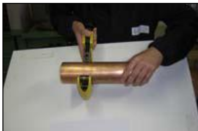
A. Cut copper tubing at right angles (using displacement type cutter or fine-toothed steel saw).
