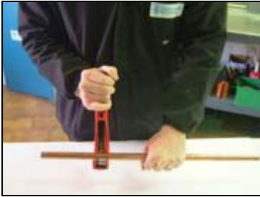
A. Cut copper tubing at right angles (using displacement type cutter or fine-toothed steel saw).
