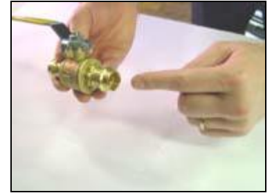
C. Check seal for correct fit. Do not use oils or lubricants. Use only the valve's black EPDM o-ring seals.
