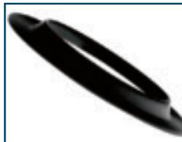
In abrasive services, deflection cones can be mounted between the upstream valve flange and the adjoining piping. Though reducing the port area slightly, they can increase the life of the seat and gate and are less expensive to replace than the entire valve. Deflection cones are available in Ni-Hard and HDPE materials.
